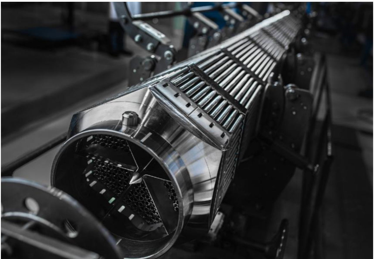
Hexagonal fuel assembly manufactured by TVEL. Credit: Rosatom's fuel company TVEL
