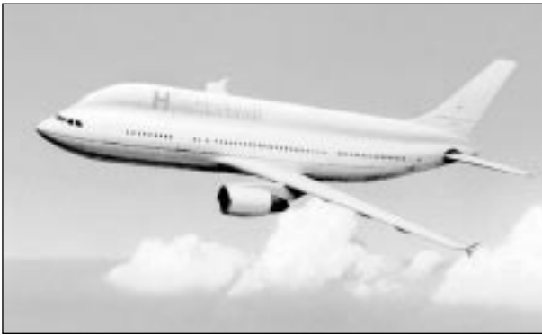
Picture 5.5: Cryoplane DaimlerChrysler's hydrogen-driven Cryoplane is based on Airbus 320
