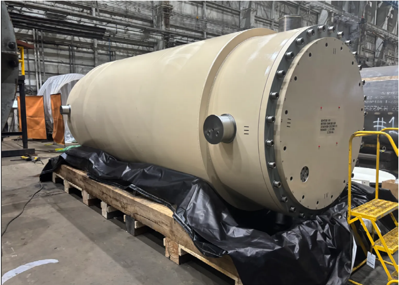
A HI-STAR 149 cask manufactured by Holtec, designed for transporting spent nuclear fuel from the spent fuel pools of VVER-1000 reactors at Kudankulam NPP units to a centralized on-site spent fuel storage facility. Source: Holtec
