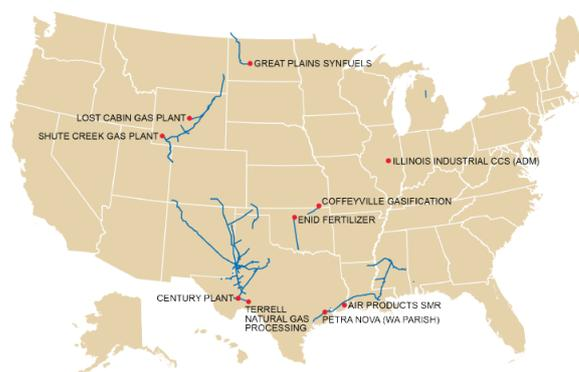
Figure ES-9. Schematic Map of CO<sub>2</sub> Pipelines in the United States
