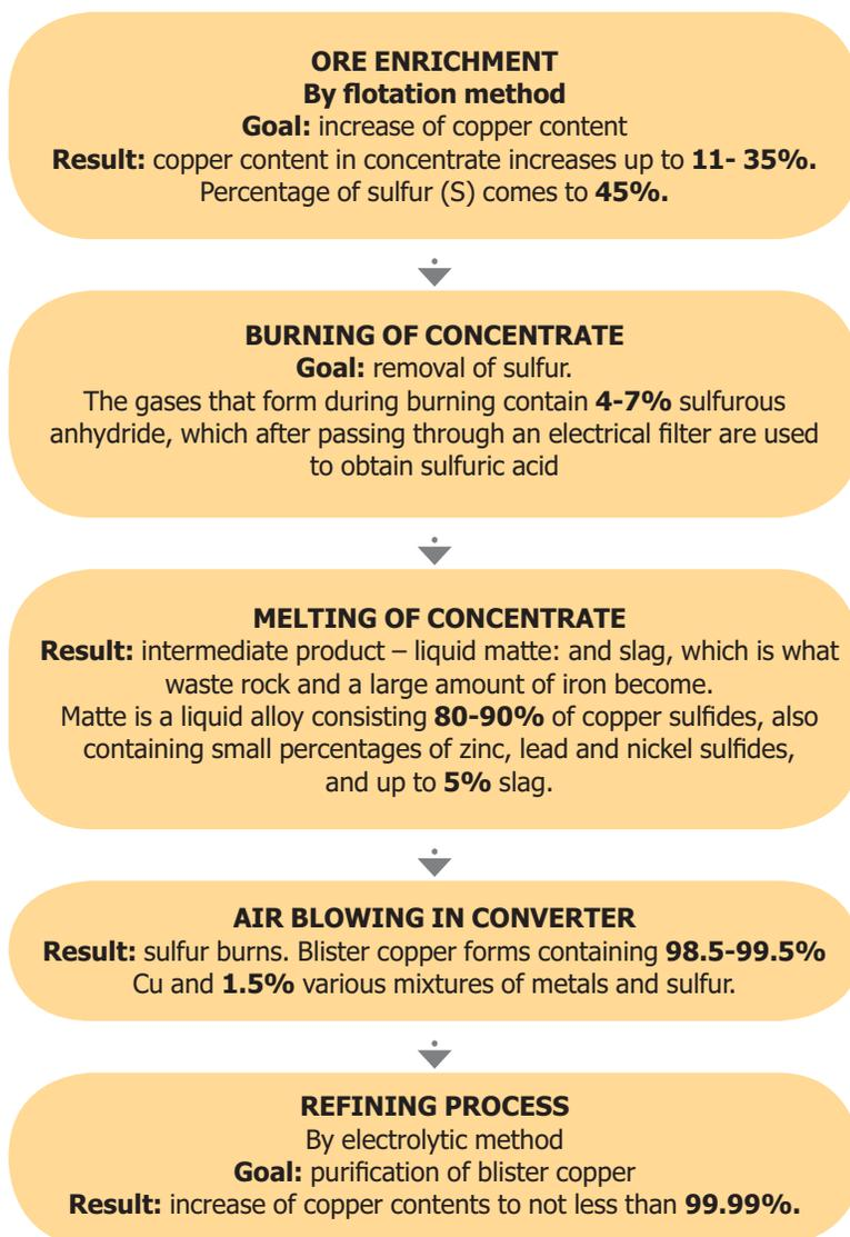
Norilsk Nickel plants use raw materials characterized by a low content of commercial components (metals). Due to this, an obligatory stage of the technological process is refinement of ore and production of concentrates, where the content of metals reaches several dozen percent.
