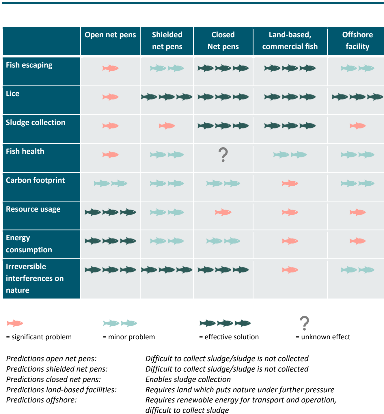
Figure 1. A comparison of the environmental impact of different technologies used during the marine phase of salmon farming. As several technologies have not yet been tested at scale, future developments, new knowledge, and more experience could influence the assessment of environmental impacts.
